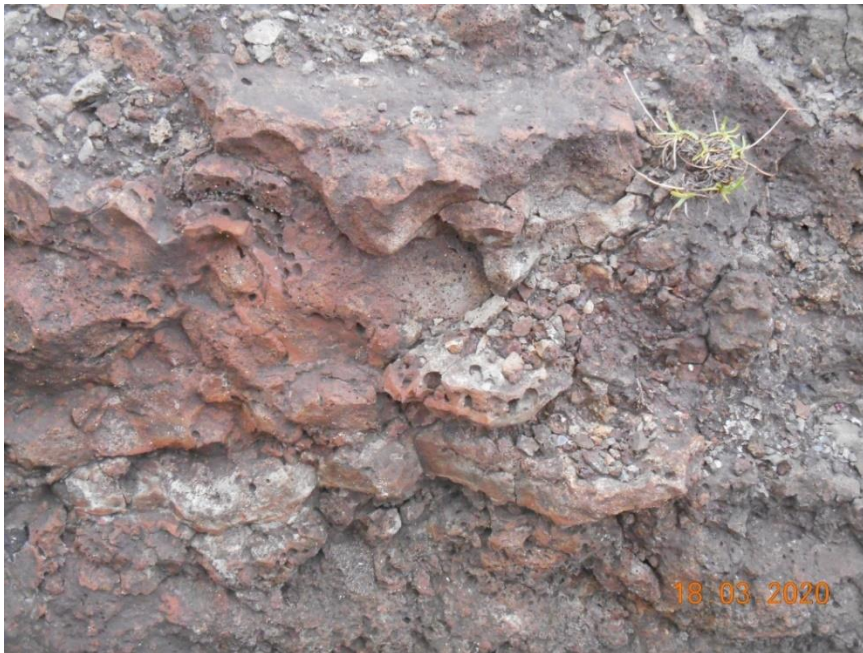
Plate 2 -Typical composition of the fused blast furnace slag.
