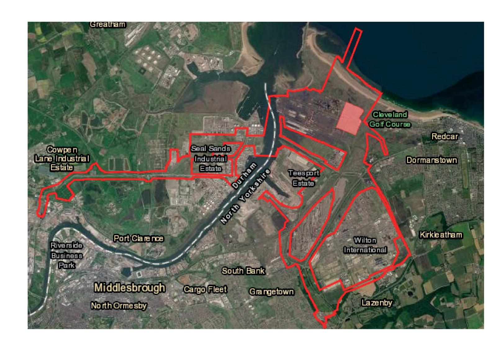
The gas-fired power station and CO, compressor station will be located on part of the former SSI steel works site in Redcar, land that is controlled by the South Tees Development Corporation. The CO, transport/export pipeline will also start in this location (minimising the distance it has to travel over land) before heading offshore. The power station connections and the CO, gathering network will involve land within both Redcar and Stockton-on-Tees, including crossings beneath the River Tees.
