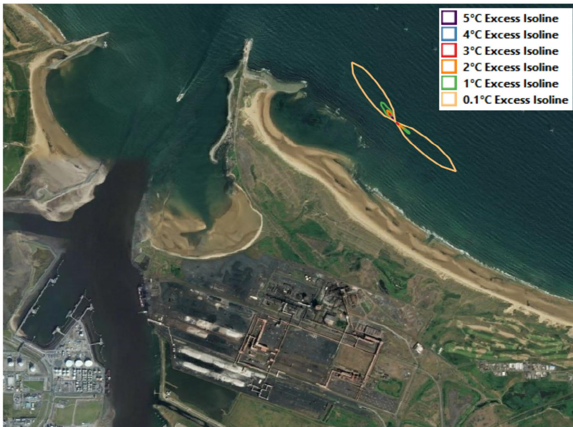
Picture 14-2: CORMIX Excess Temperature Isolines (°C) Under Mean Spring, Peak Flood (Southeast) and Ebb (North West) Tidal States
